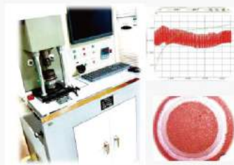
Tribometer Force 10kN
