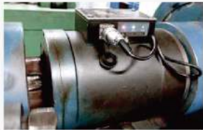
Test Rig for oscillating movements, Force 615kN
