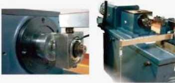
Rotating Test Rig PV-Evaluation, Force 35kN
