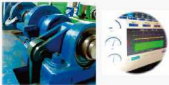
Test Rig for oscillating movements, Force 615kN
